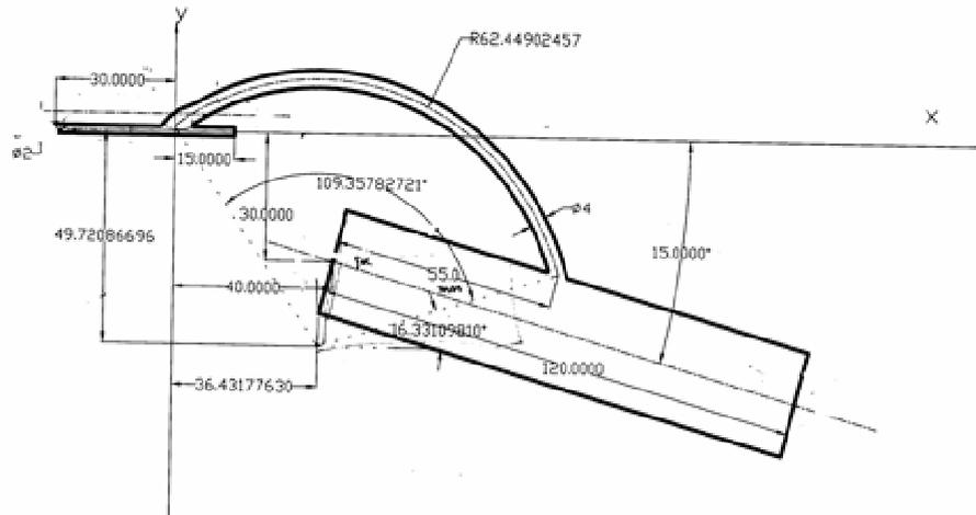
Figure 3a Geometry & dimensions (mm) of the coronary arterial bypass graft system
