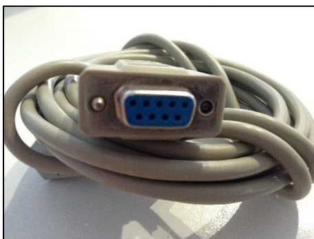
Fig 2. Female RS-232 Connector
