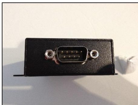
Fig 1. Male RS-232 Connector
