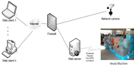
**Fig. 3** Conceptual framework outlining the various components (subsystems) and their interaction in the proposed web-based manufacturing system [8].
