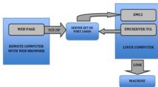
Fig. 2 Schematic Representation of WEB Control of Machine [5]
