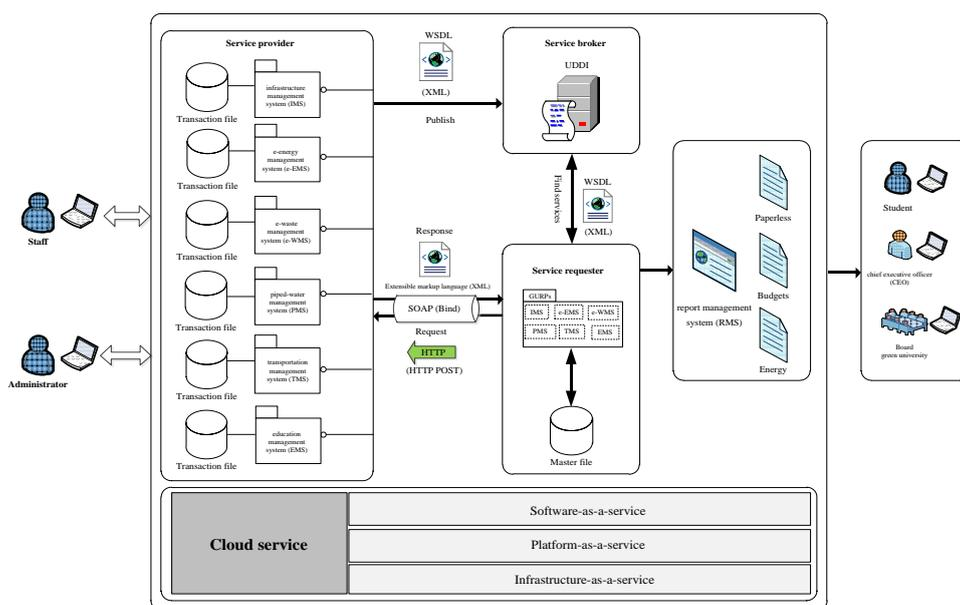
Fig. 2 The System Architecture of GURP on Cloud Computing.
