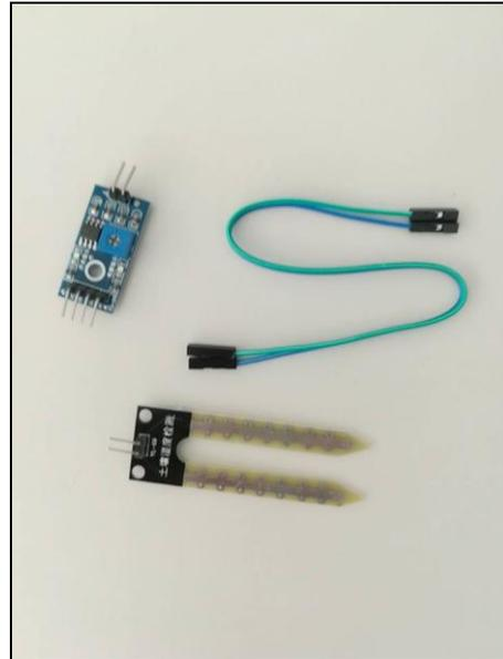
Fig. 3 Soil Moisture Sensor
