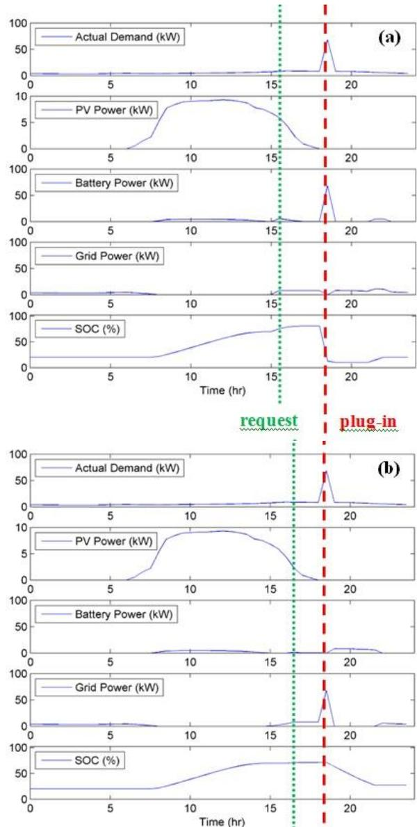
Fig. 2 System's Power Profile when Request for Quick Charge 3 hr. in Advance (a) and 2 hr. (b)
