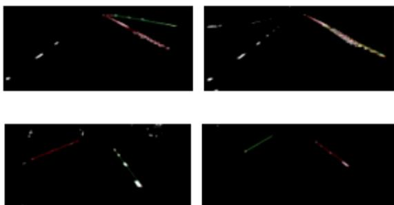
**Fig. 7** Lane Detection Results by Hough Transform
