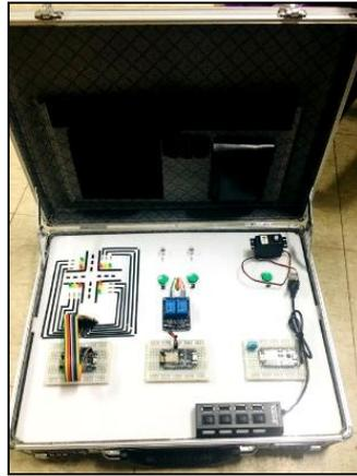
**Fig. 1** Experimental Set of Electrical Traffic Signals Controlled
