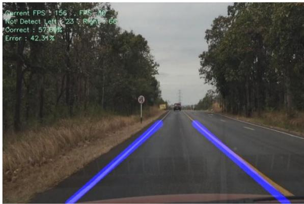
Figure 8. Find Lane Used by Hough Transform
