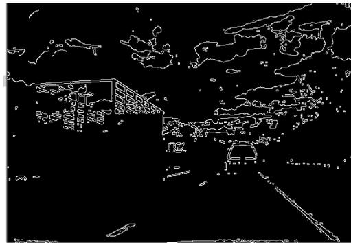
Figure 7. Finding Edge by Canny Algorithm
