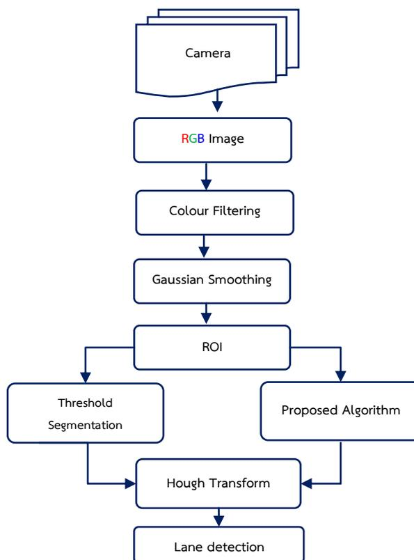
Figure 2. Flow Diagram of the Lane Detection
